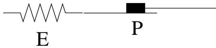
Fig. 7. An elastic element and a plastic element connected in series.
