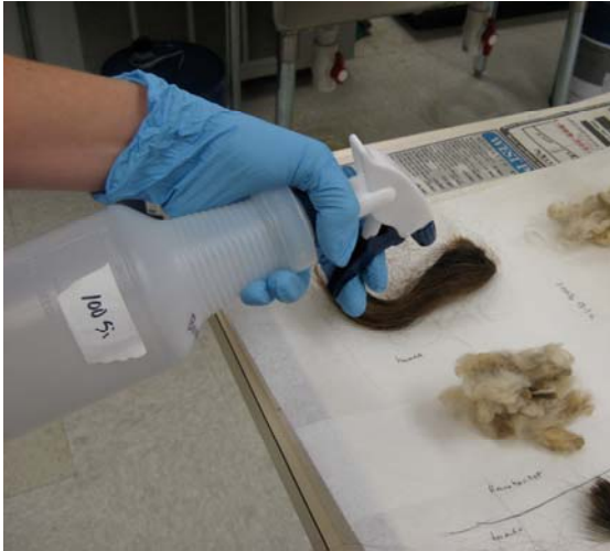
Figure 13. Spray application of 100% silicone oil to samples
