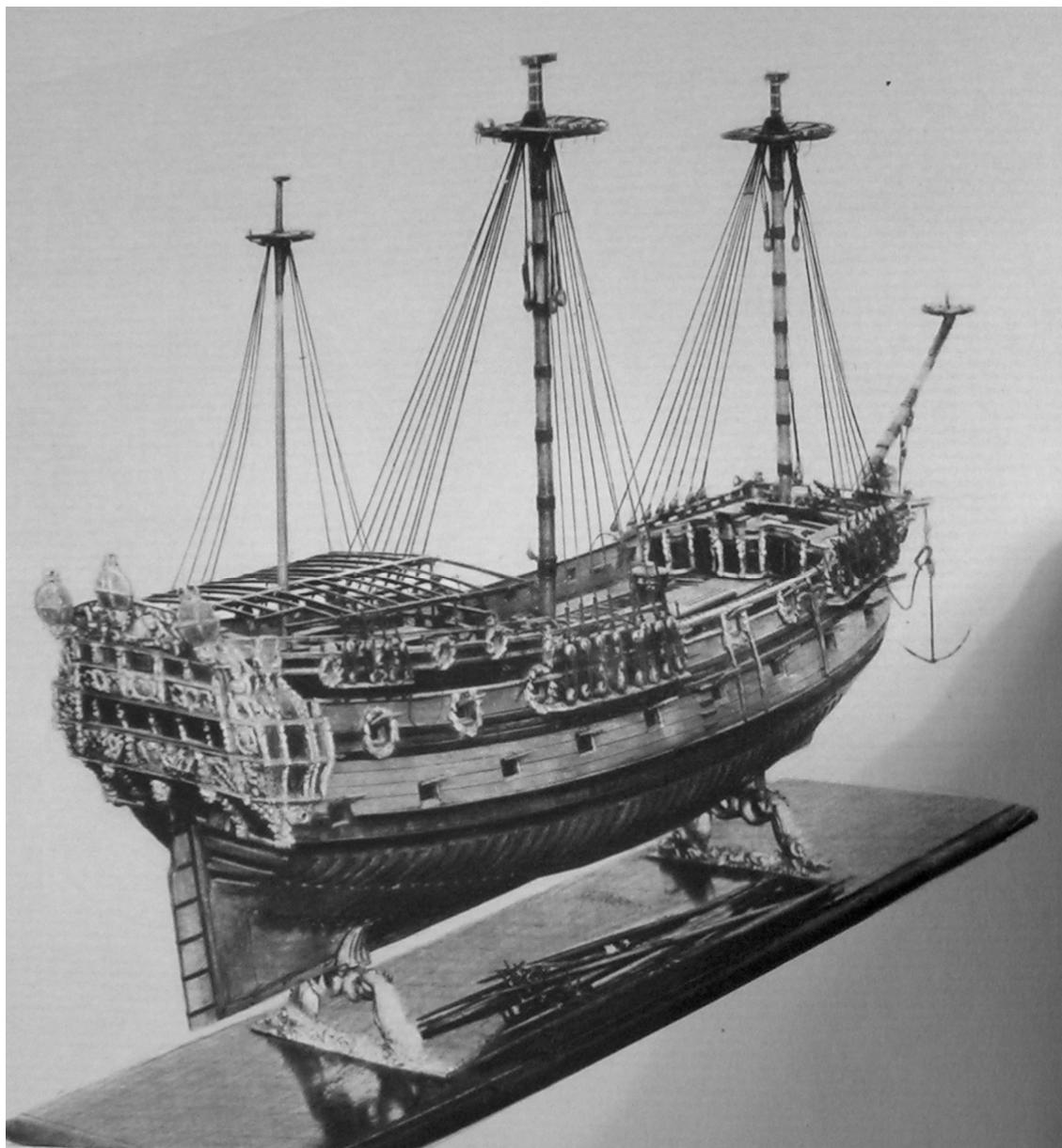
Fig. 41. Unidentified fourth rate 48-gun warship. The rigging seems to be contemporary with the hull. Notice the framing on top of the stern castle for a canvas awning. (From Culver 1954, 36)
