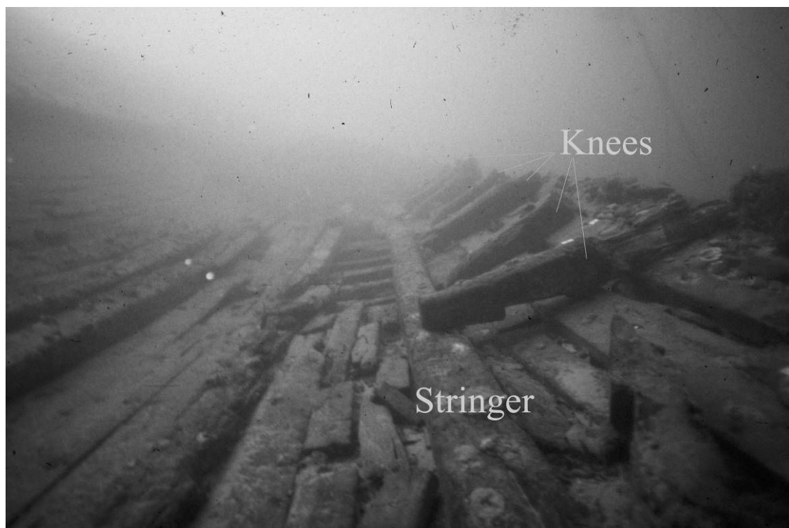
Fig. 96. Photograph of the port side dormente dos baileus and hanging knees, facing aft. (Courtesy Robin Percy)
