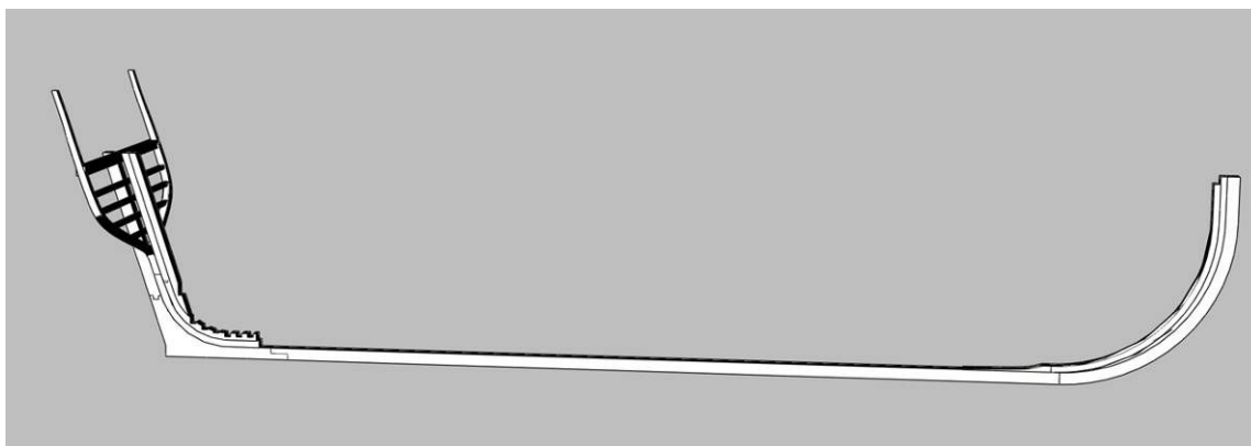
Fig. 77. Keel and ends of the vessel.
