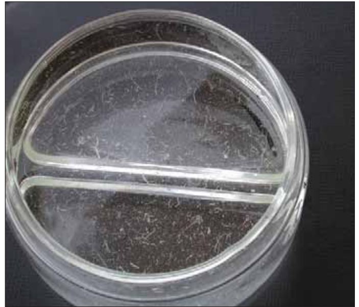
Figure 6. Worms flushed from an SDI system. Flushing twice a week solved the problem.
