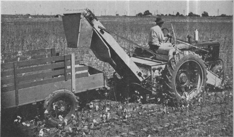
Figure 2. Rear view showing tractor-mounted extractor unit. Used in combination with the stripper-harvester.
