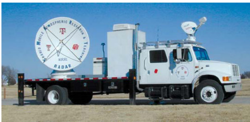
FIG. 3.1. Photograph of SR1. Truck cab represents area of beam blockage (Biggerstaff et al. 2005)
