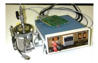
Fig.2.3. RSST including a pressure vessel and control unit (http://www.chem.mtu.edu/~crowl/rsst.htm)
