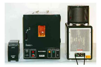
Fig.2.5. RADEX cell (left), SEDEX cell (middle), and SIKAREX cell (right) (http://www.systag.ch/e530tsc5.htm# Measuring\_cells)
