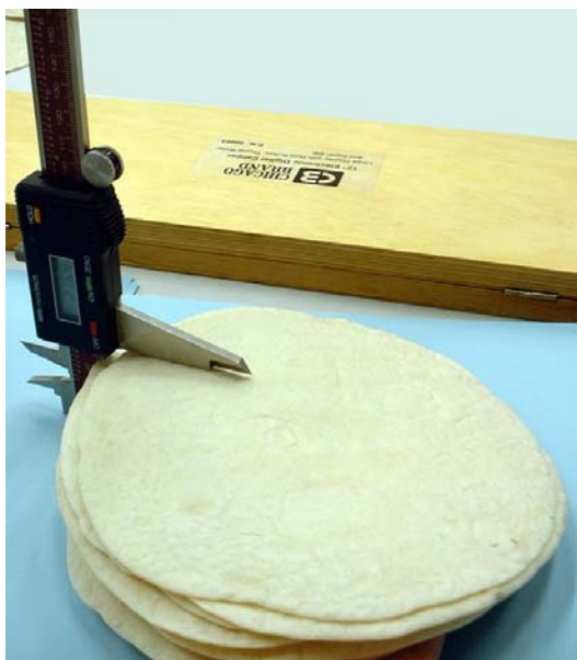
Fig. C.1. Measurement technique for height.
