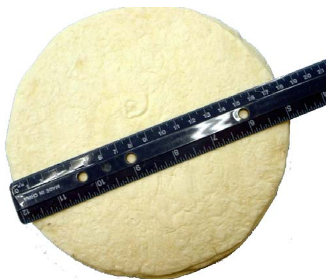
Fig. C.2. Measurement technique for diameter.
