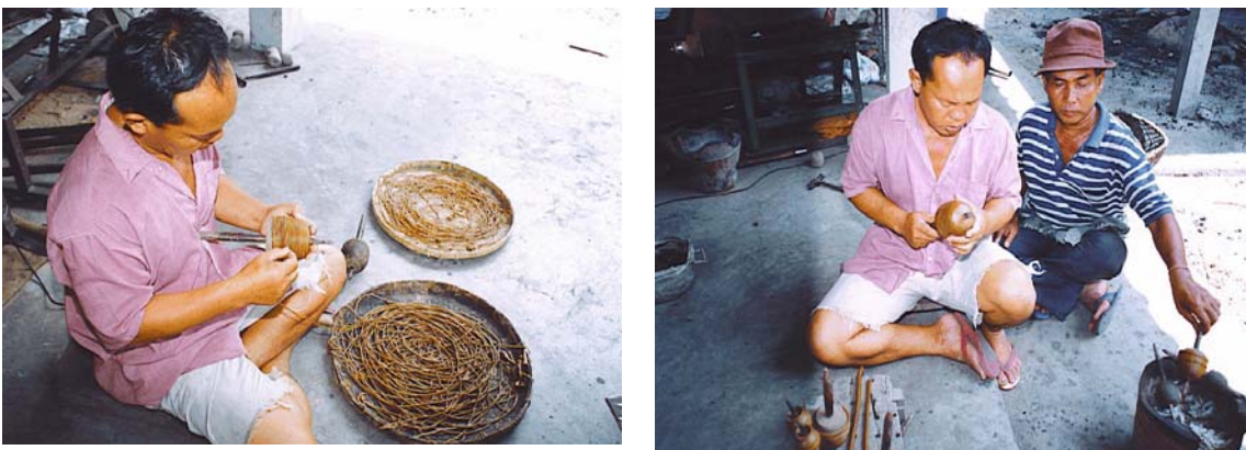
Figure A-11. Wax coating of the inner moulds.
