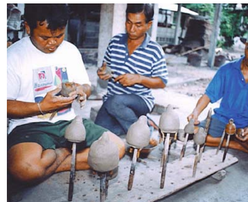
Figure A-14. Sealing the wax coated moulds.
