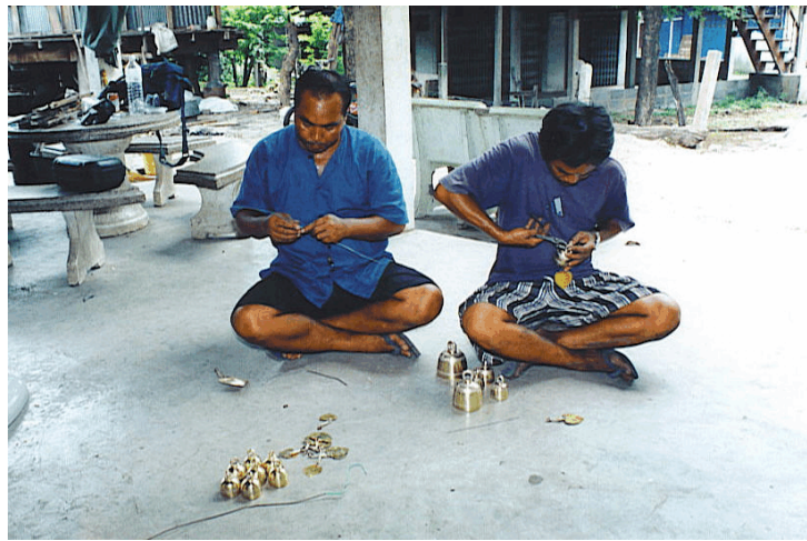
Figure A-25. Attaching the clapper and wind fan to the bell.
