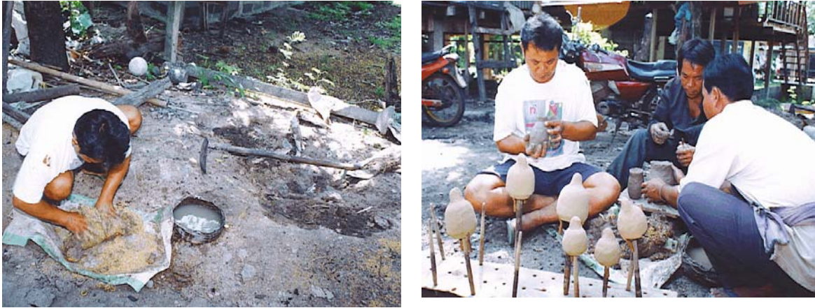
Figure A-15. Applying the external moulds.
