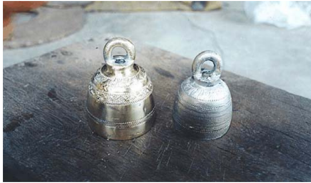
Figure A-24. Comparison of a polished and unpolished bronze bell.
