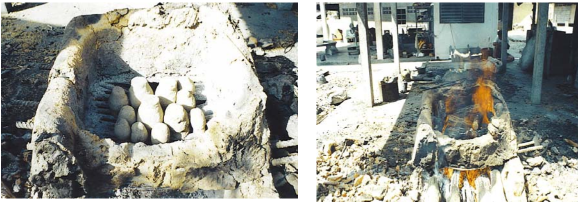
Figure A-16. Melting the wax from the moulds.
