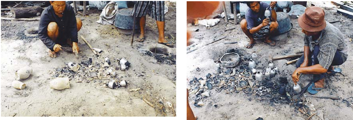
Figure A-21. Removing the bronze bells from the clay moulds.
