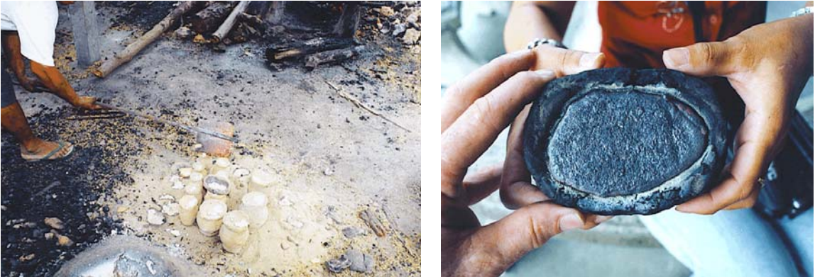
Figure A-20. Making an ox-hide bronze ingot.
