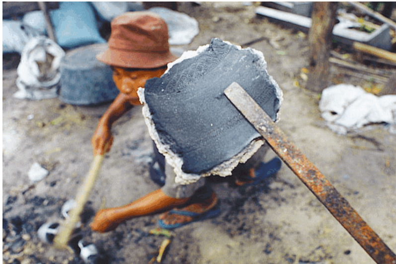
Figure A-26. Vitrified inner portion of external clay mould.
