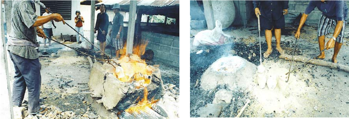
Figure A-19. Pouring the bronze into the moulds.
