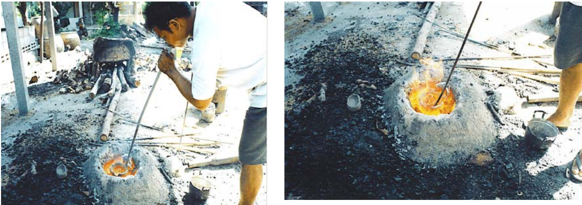
Figure A-18. Heating the bronze in a crucible set inside a bowl furnace.
