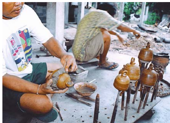
Figure A-14. Sealing the wax coated moulds.
