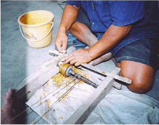
Figure A-12. Preparing the wax coated moulds for the appliqué.
