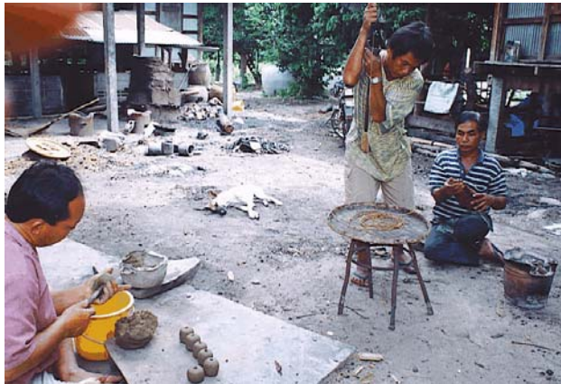
Figure A-10. Making wax string with a chest press.
