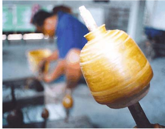
Figure A-12. Preparing the wax coated moulds for the appliqué.
