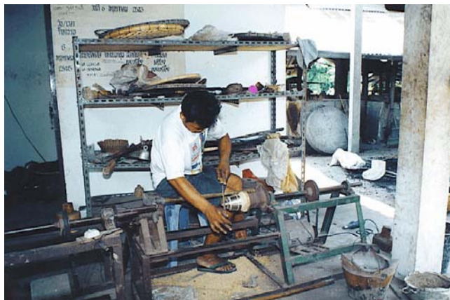
Figure A-23. Polishing the bell on a lathe.
