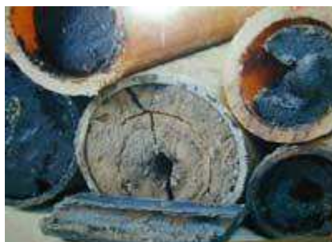
Fig. 1. Reduction in internal diameter of pipeline [1]
