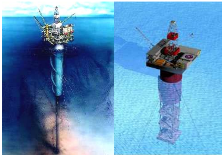
Fig. 1.2. Example Pictures of classical spar (left) and truss spar (right) (Courtesy, J. Ray McDermott).
