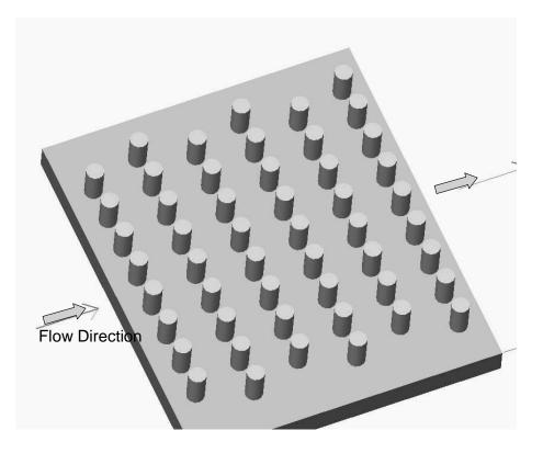
Fig. 1. Typical Pin Fin Configuration
