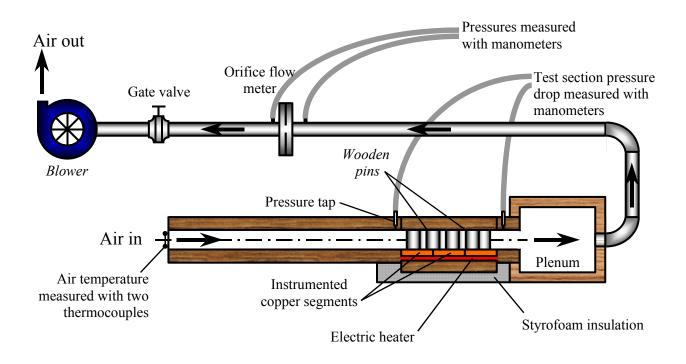
Fig. 3. Layout of the Experimental Setup
