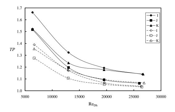
Fig. 9. Effect of H/D on Thermal Performance for D = 2.54cm
