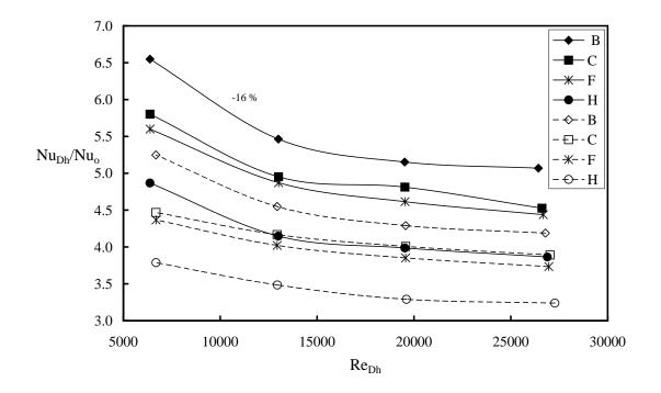
Fig. 4. Effect of  $Re_{Dh}$  on Heat Transfer Enhancement for D = 1.27cm
