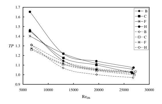
Fig. 6. Effect of  $Re_{Dh}$  on Thermal Performance for D = 1.27cm
