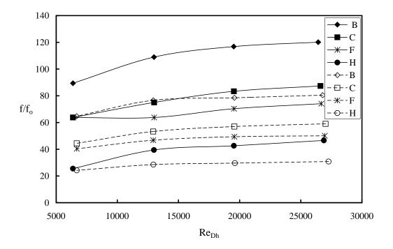
Fig. 5. Effect of  $Re_{Dh}$  on Increase of Overall Pressure Drop for D = 1.27cm
