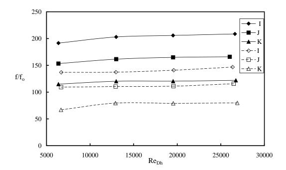
Fig. 8. Effect of H/D on Increase of Overall Pressure Drop for D = 2.54cm
