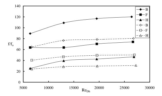
Fig. 14. Effect of  $S_T/D$  on Increase in Overall Pressure Drop for D = 1.27cm
