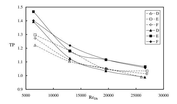
Fig. 12. Effect of  $S_L/D$  on Thermal Performance for D = 1.27cm
