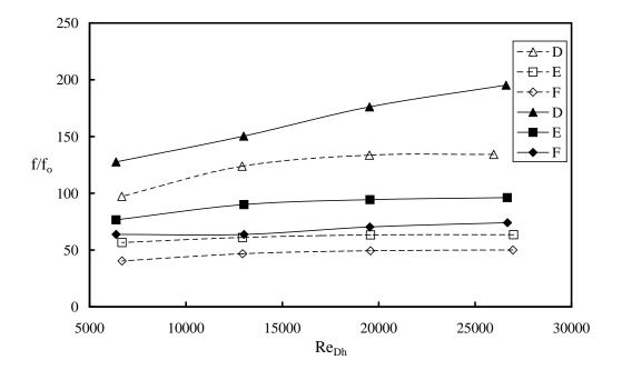
Fig. 11. Effect of  $S_L/D$  on Increase of Overall Pressure Drop for D = 1.27cm
