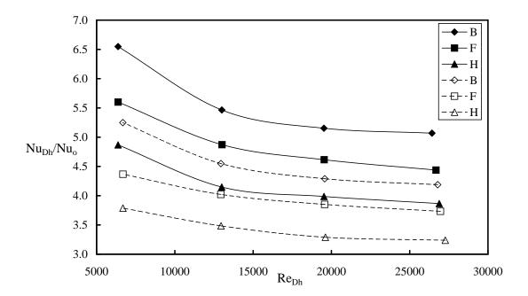
Fig. 13. Effect of  $S_T/D$  on Heat Transfer Enhancement for D = 1.27cm
