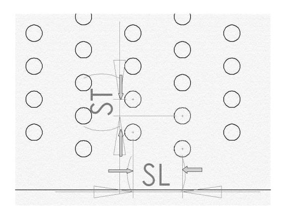
Fig. 2. Streamwise  $(S_L)$  and Transverse  $(S_T)$  Distances of a Pin Fin Configuration
