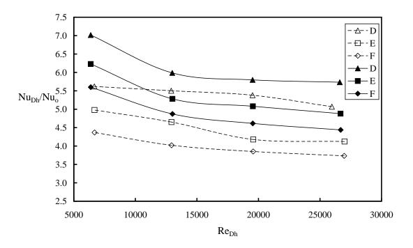
Fig. 10. Effect of  $S_L/D$  on Heat Transfer Enhancement for  $D{=}1.27\text{cm}$
