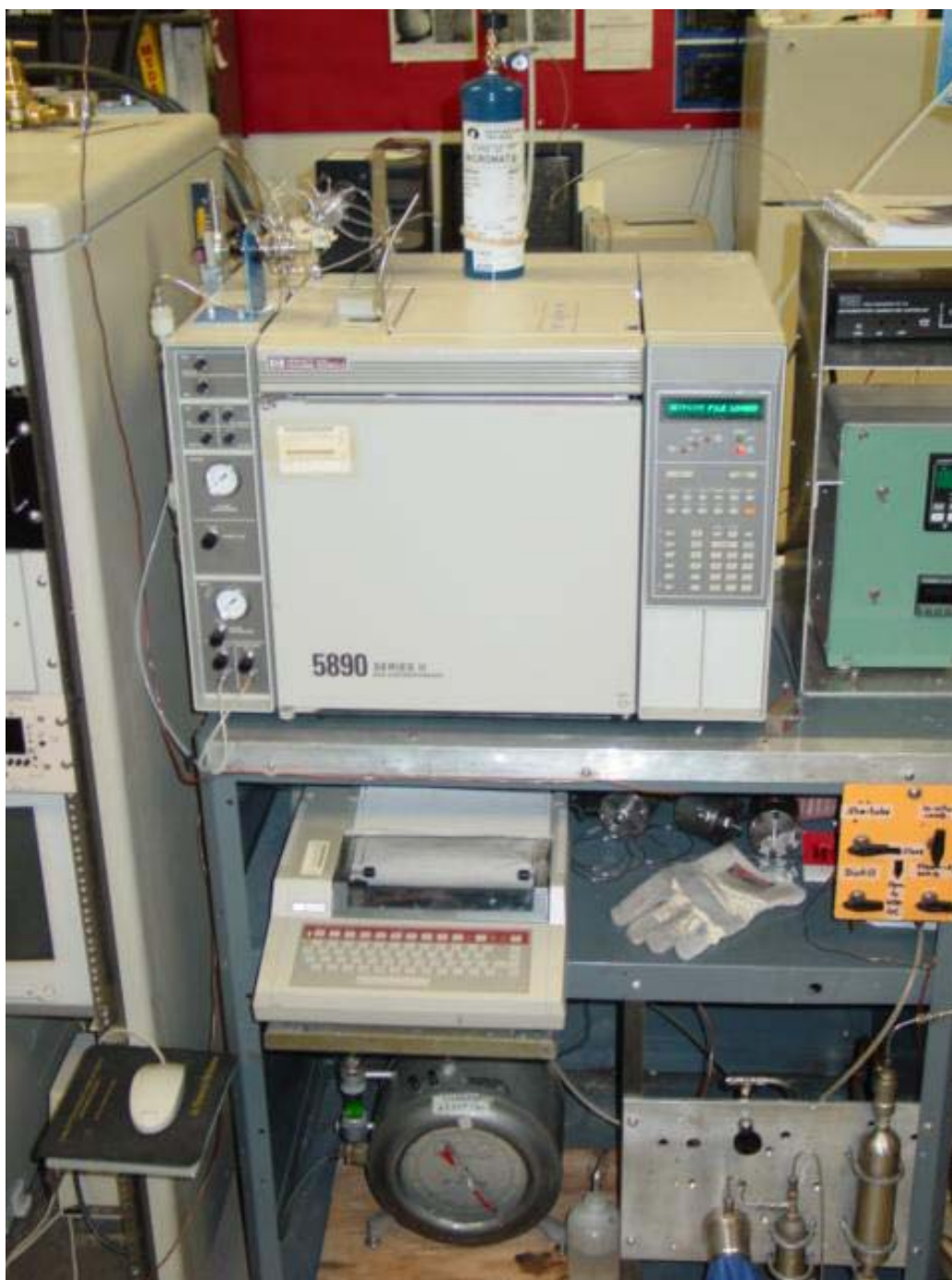
Fig. 3.10—HP 5890 Series II gas chromatograph and wet test meter.
