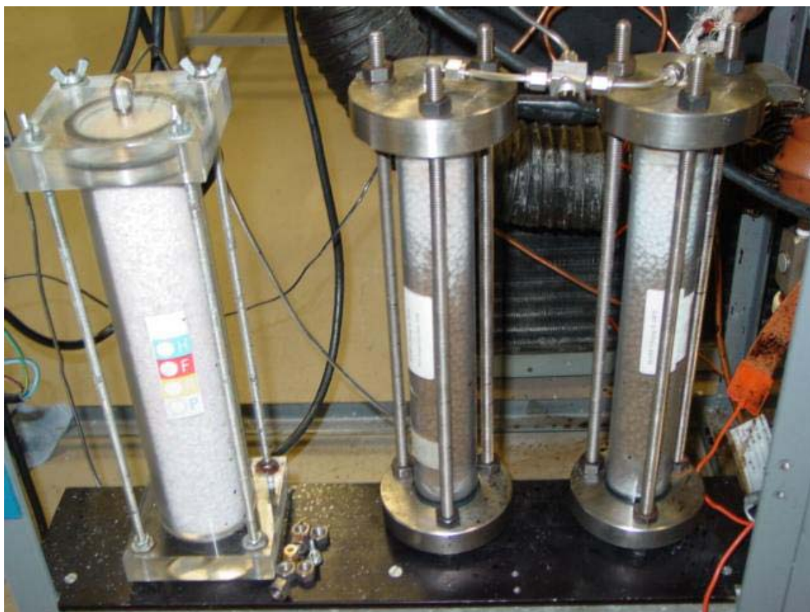
Fig. 3.9—Acid scrubber and drierite columns.
