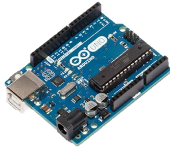
Figure 30. Arduino UNO revision 3 board used for sensing coil voltage measurement and control of actuators [35]
