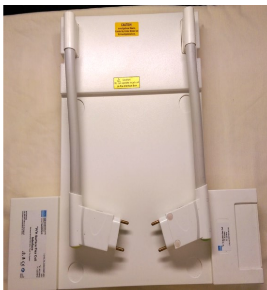
Figure 16: Interface box which corresponds with the ^{31}\text{P}/^1\text{H} commercial coil
