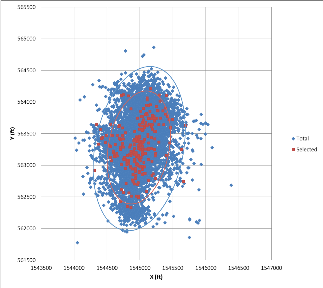
Figure 18. Map view of all Well A events and high SNR, high magnitude events
