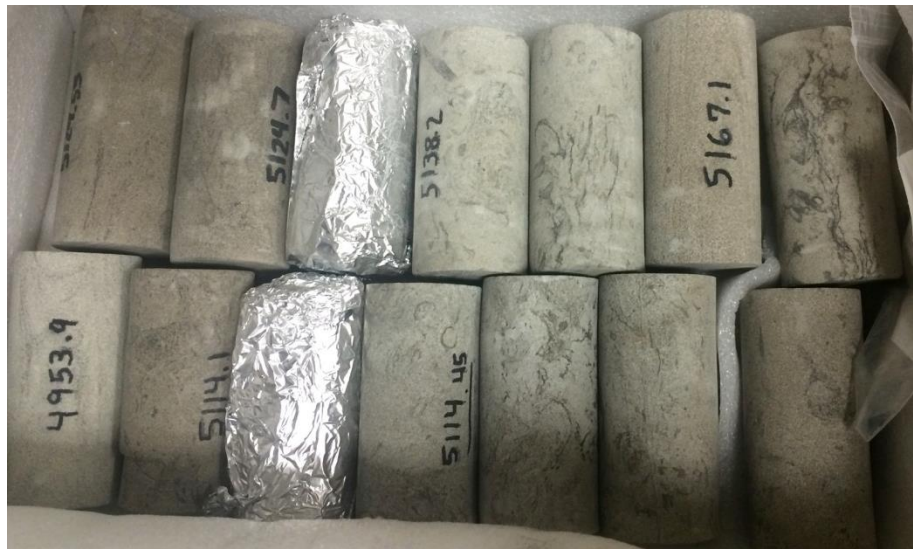
Fig. 32—Figures of Katz cores from KSU 326 and KSU 231 in the size of 1.5 in. × 3 in.
