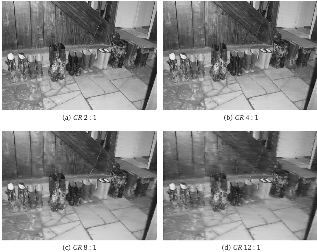
Figure 7.16. Compressed images of Figure 7.4c applying increasing compression rates CR = 2, 4, 8, 12 . In order to reconstruct the images we exploit all the coefficients of the 3 levels tree and we use the new matrices in (7.41).
