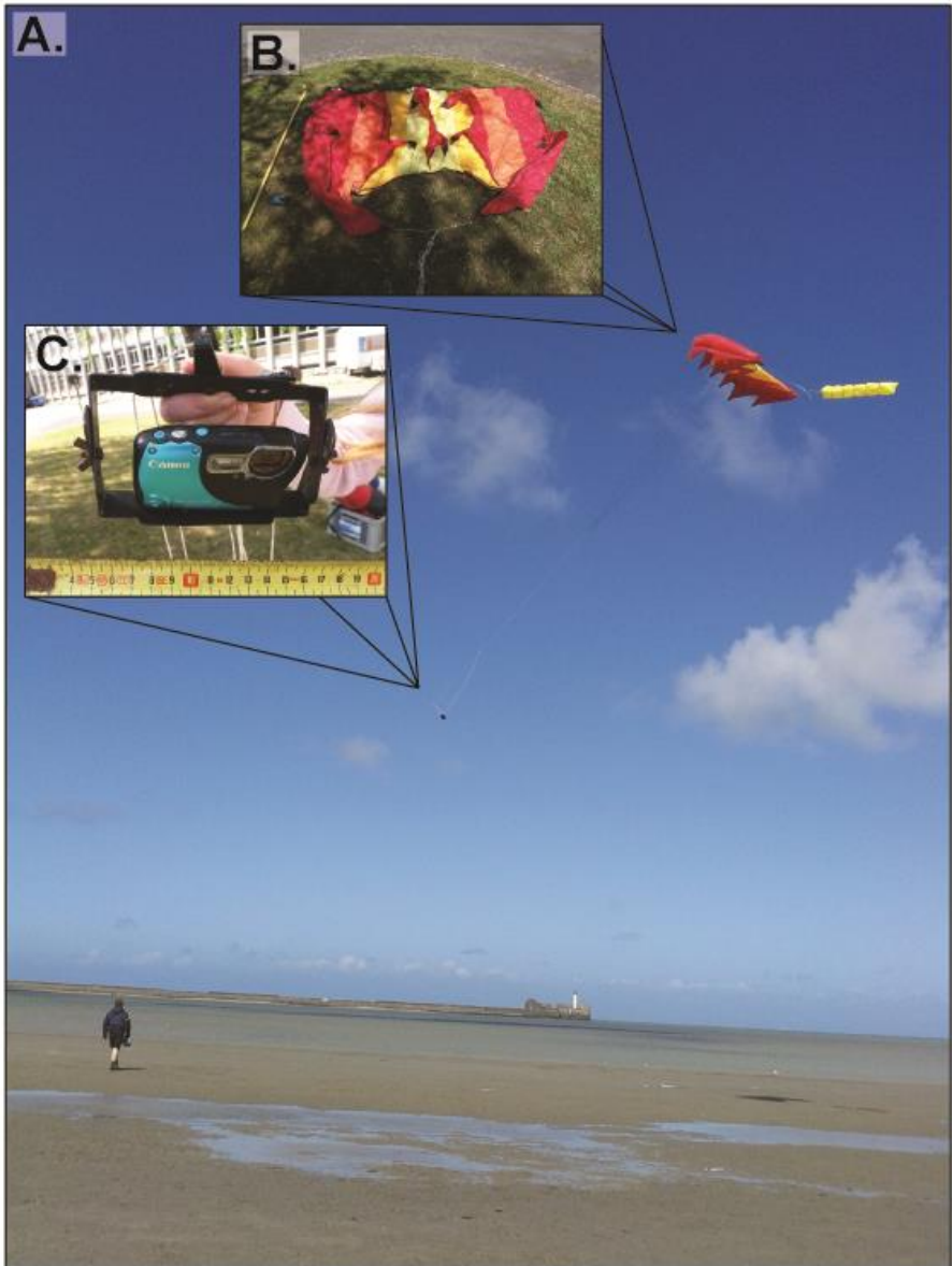
Fig 4.2. Kite pilot mapping the study site (A) with the Flowform kite (detail in B) mounted with a mechanical picavet suspension carrying a Canon PowerShot D20 digital camera (detail in C).
