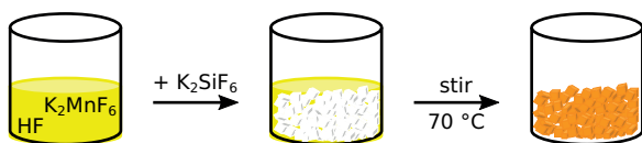
Figure 9.1: Schematic illustration of the cocrystallization synthesis where \text{K}_2\text{SiF}_6:\text{Mn}^{4+} is formed from \text{K}_2\text{MnF}_6 and \text{K}_2\text{SiF}_6 in a slurry.
