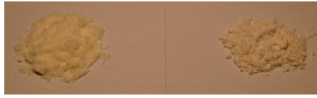
Figure 7.5: Body color of \text{K}_2\text{SiF}_6:\text{Mn}^{4+} from a precipitation synthesis at 0^\circ\text{C} without (left) and with bubbling through \text{N}_2 (right) during the synthesis.
