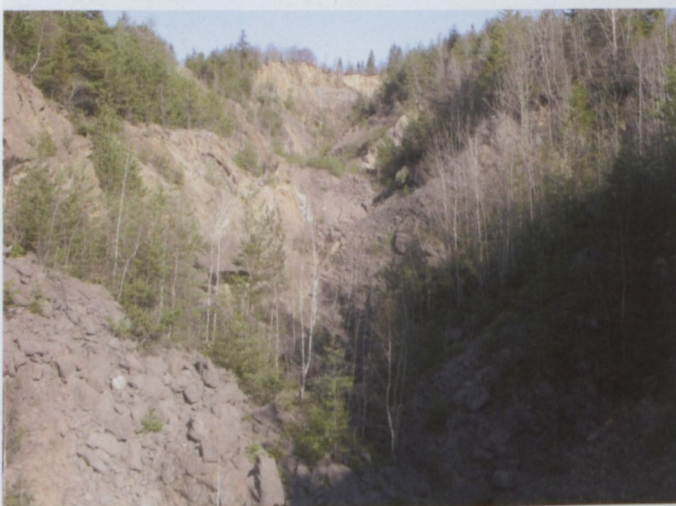
Fig. 29. One of several abandoned open pits excavated in the uppermost part of the Droždiak siderite-barite vein, south of Poráč village. The documented quarry is 50 m wide and 230 m long, but the Droždiak vein crops out here in the total length of 1 km.
