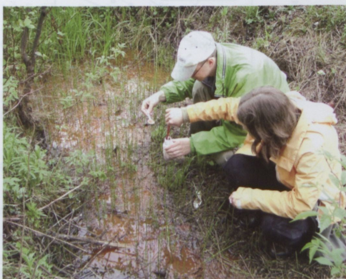
Fig. 23. Iron ochre (mainly ferrihydrite) precipitating from water outflows from tailing impoundment near Čučma.
