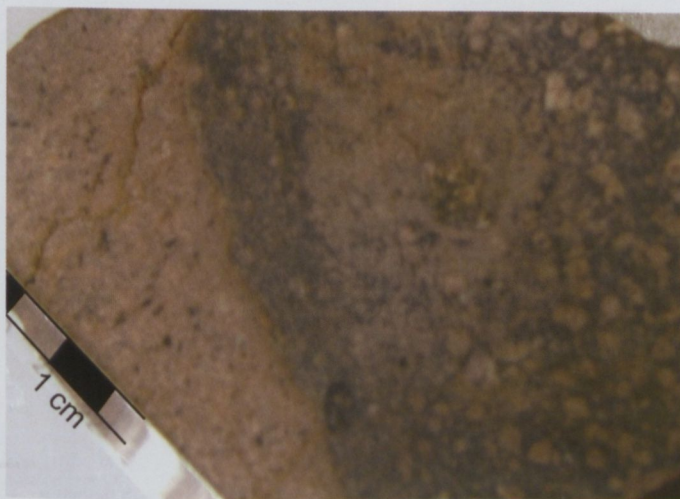
Fig. 34. Macroscopic image of the contact between the host granodiorite (left, pink) and the microgranodiorite dyke (right, dark grey) in the Cerbia outcrop (Field stop 10).
