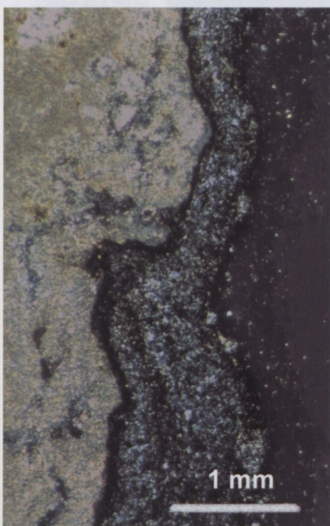
Fig. B4. Folded surface of black gypsum crust on the Upper Jurassic limestone; Kraków, City Walls.
