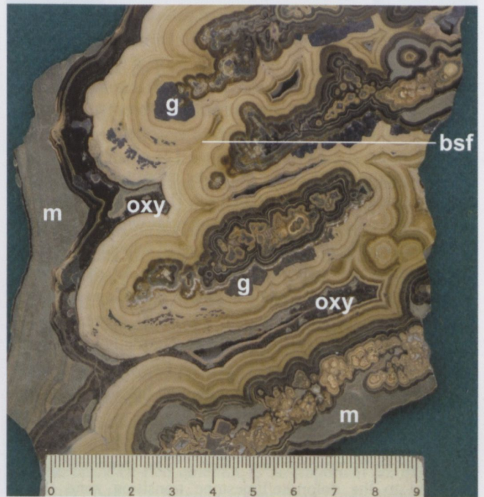
Fig. D16. Banded mineralization composed of banded ZnS (yellowish to brown), bleached sphalerite (bsf), galena (g), Fe-Zn-Pb-oxysulphides (oxy), and marcasite (m). Pomorzany mine.
