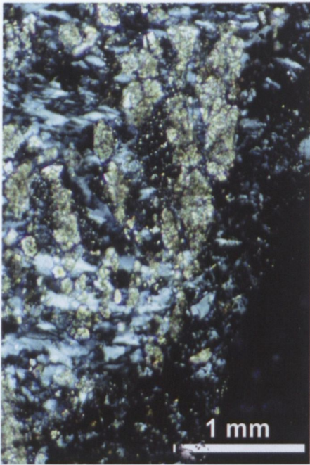
Fig. B14. Gypsum-rich outer layer of the Libiąż dolomite; wall near the Vistula River (Kraków).
