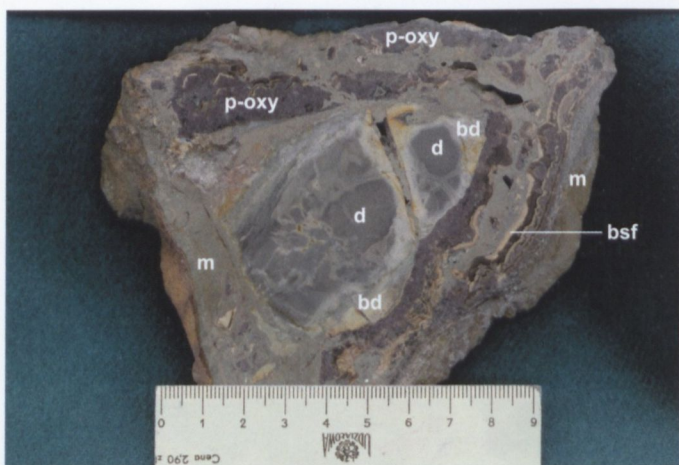
Fig. D18. Breccia ore composed of dolomite clasts (d) bleached alongside edges (bd), and overgrown by black sphalerite, bleached sphalerite (bsf), pyrite and oxysulphides (p-oxy), and marcasite (m). Pomorzany mine.
