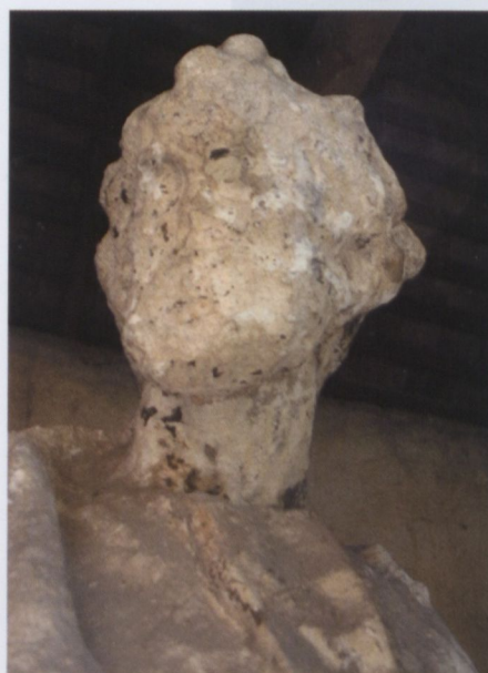
Fig. B8. Deep disintegration of the Pińczów limestone; head of an Apostel from the St. Peter and Paul Church, Kraków.
