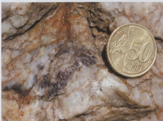
Fig. 14.2. Cassiterite aggregate (dark brown) in quartz, Dlhá dolina valley. Photo: P. Uher.
