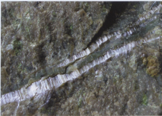
Fig. 13.2. Chrysotile veinlets in serpentinite, up to 1-2 mm in thickness, Dobšiná. Photo: P. Uher.
