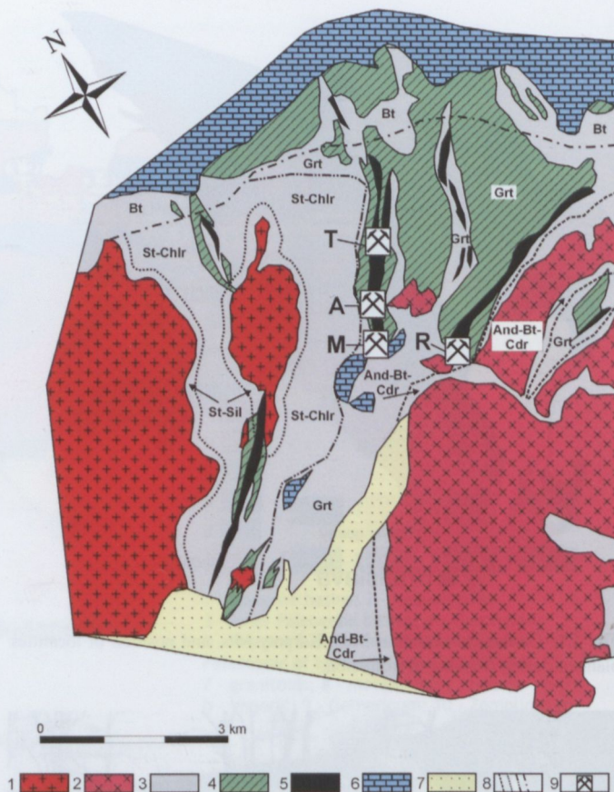
Fig. 2.1. Schematic geological map of the Pezinok-Pernek area in the Malé Karpaty Mts. (Cambel & Viliňovič 1987, adapted). 1 - Bratislava granitic massif; 2 - Modra granitic massif; 3 - metapelites; 4 - metabasic rocks; 5 - pyrite-pyrrhotite-enriched metabasic rocks (1 to 5 Paleozoic); 6 - Mesozoic sedimentary rocks; 7 - Cenozoic sedimentary rocks; 8 - metamorphic isogrades; 9 - pyrite-pyrrhotite deposits with V-Cr mineralization: Rybníček (R), Trojárová (T), Augustín (A) and Michal (M).
