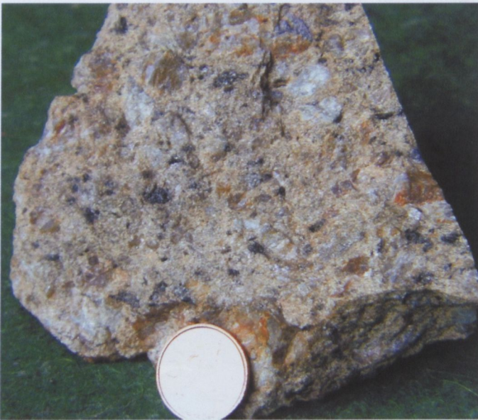
Fig. 15.2. Porphyritic granite (granite porphyry), typical main intrusive rock of Betliar area. Photo: M. Kubiš.
