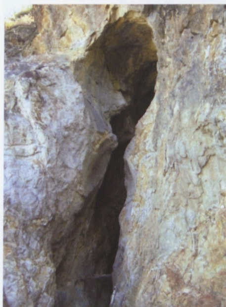
Fig. 16. The entrance in the Roman stope from Găuri mining field (Cetate massif). The stope shows typical rounded walls in the upper part while in the lower part it was re-shaped by the modern exploitation (traces of blast holes). The width of the stope is about 1.8 m at the bottom of the image (Photo C. Tămaș).
