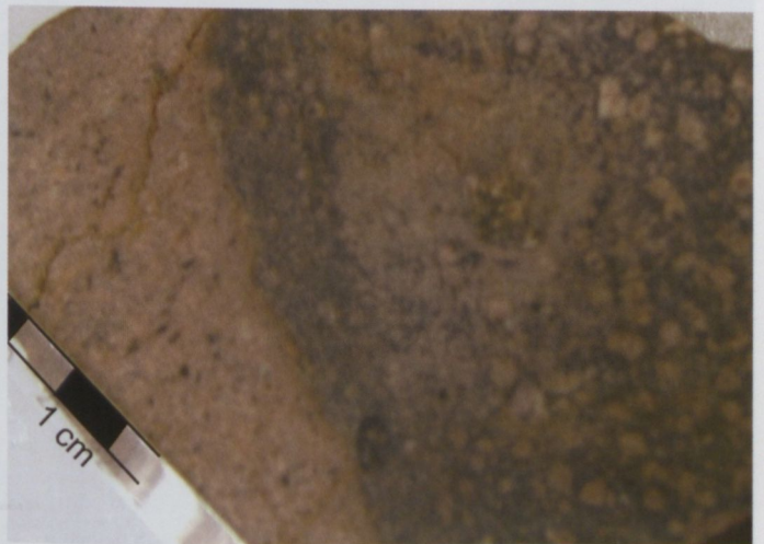
Fig. 34. Macroscopic image of the contact between the host granodiorite (left, pink) and the microgranodiorite dyke (right, dark grey) in the Cerbia outcrop (Field stop 10).
