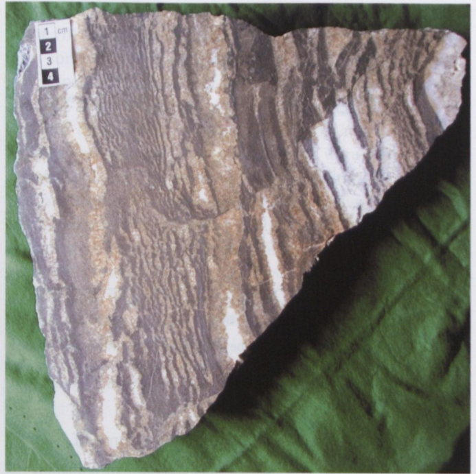
Fig. 13. “Tiger-type ore”, showing banding of siderite, white ankerite and grey layers rich in fine-grained pyrite, organic matter, quartz and sericite.
