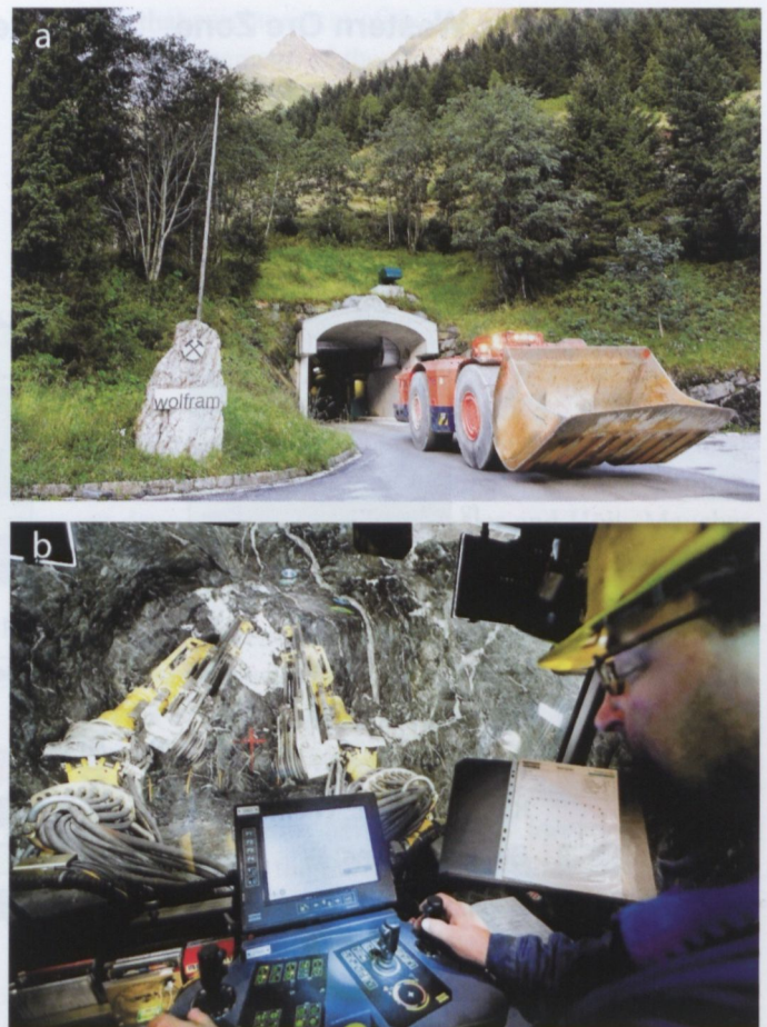
Fig. 17. a) Portal of the Felbertal underground mine. b) Drilling with modern computer-controlled two-boom jumbo.
