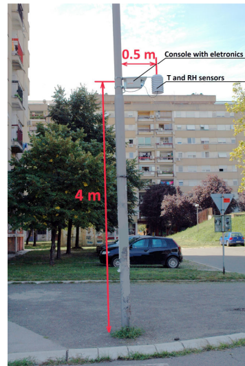
Fig. 5 Example of monitoring network station in Novi Sad (Serbia) mounted on a lamppost (Šećerov et al. 2015b)
