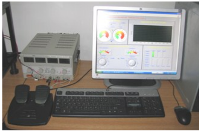
Figure 3 The accelerator pedals and the front panel of the application with LabVIEW interface
