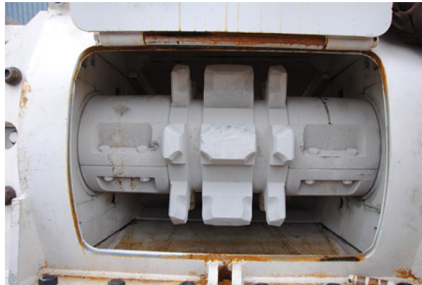
Figure 2. Chain drum installed in an armoured face conveyor
