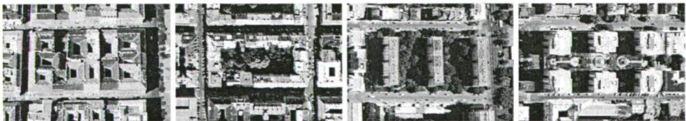
Fig. 1 From left to right: the block of courtyard apartments, the perimeter block, the Zeilenbau configuration and the hybrid block typology (Google Maps 2010)
