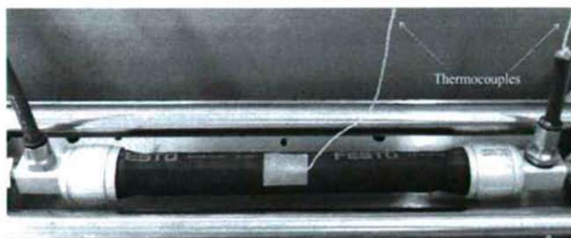
Figure 1. Muscle with two thermocouples
