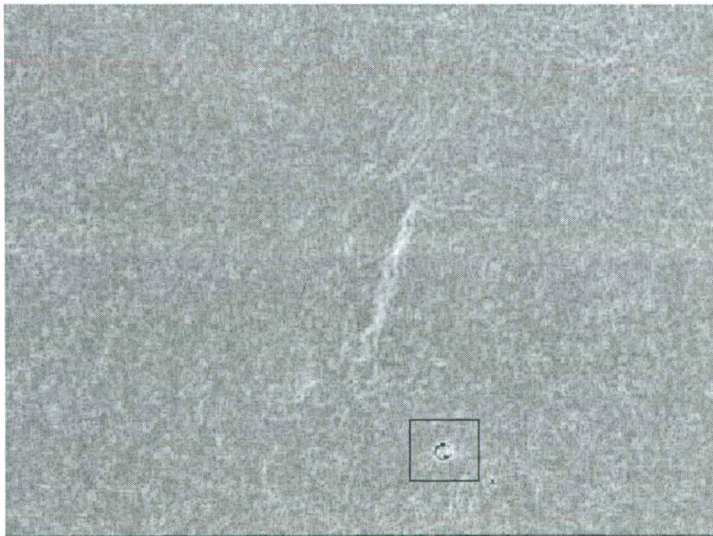
Figure 13. The image on Fig. 11. further filtered with a Sobel filter (darker spot marking the site of leakage)
