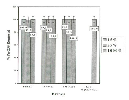
**Fig. 1:** Percentage of <sup>239</sup>Pu removed from brines after equilibrated with MgO backfill for 68 days.
