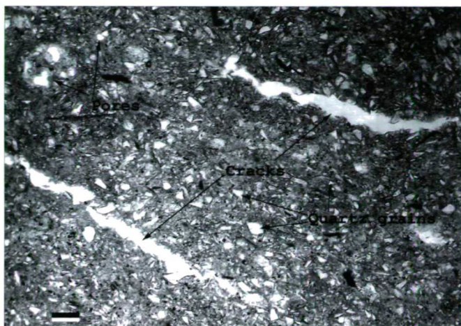
Fig. 5. Microstructure of the ceramics (1300 °C) (NII, 0.125mm bar).
