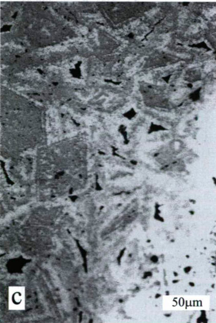
Fig.5a. Hexagonal-shaped goethite and jarosite pseudomorphs after pyrite. Fig.5b. Rhomb-shaped goethite pseudomorphs after marcasite. Fig.5c. The older goethite generation of boxwork texture. Fig.5d. The younger goethite generation of colloform texture.
