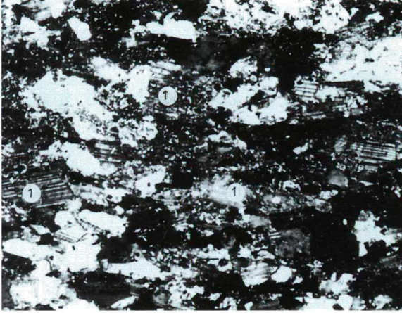
Fig. 3. Meladiorite with textural ordering Striped arrangement of plagioclase crystals (x23; +N)
