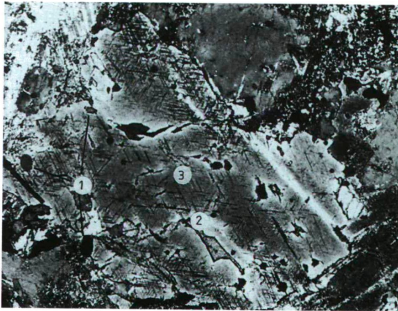
Fig. 6. Meladiorite with textural ordering Hornblende(3) with apatite(1) and calcite(2) inclusions (x23; +N)
