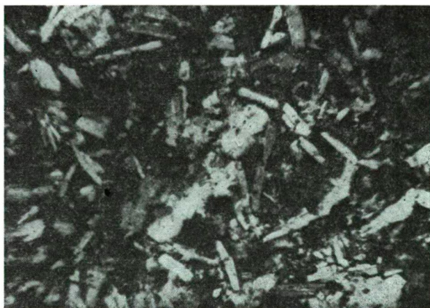
Fig. 11. Photomicrograph of spilite, composed of albite laths displaying intersertal texture in a chloritic groundmass. Crossed nicols, 20\times .
