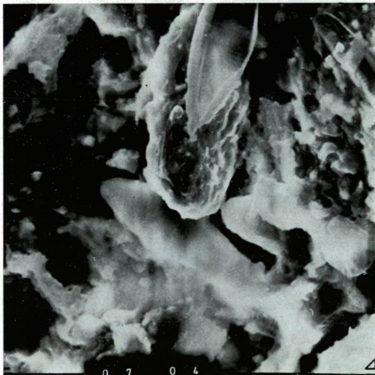
Fig. 6. Oil shale. Surface picture with diatome skelets. SEM 3000 X. Record by K. PINTYE—HÓDI. Bore Put—7: 16.0—16.5 m.
