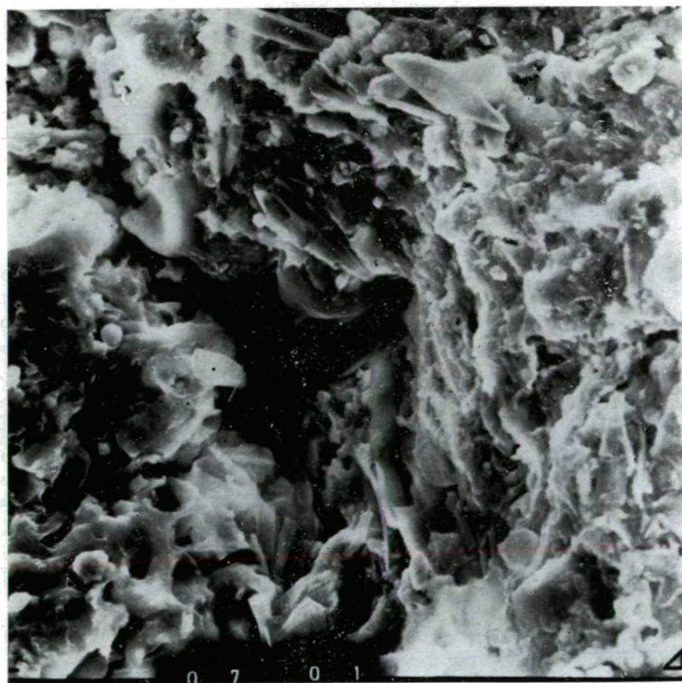
Fig. 5. Oil shale. Surface picture. SEM 1000 X. Record by K. PINTYE—HÓDI. Bore Put—7: 16.0—16.5 m.
