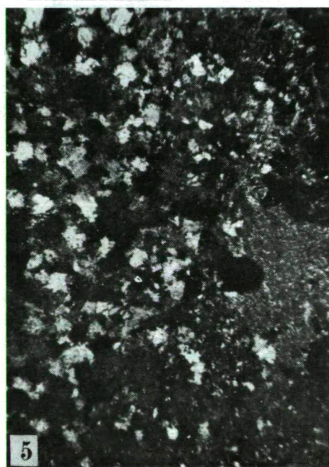
Fig. 2. Sericitized feldspar. +N X 80. Fig. 3. Idiomorphic chloritized pyroxene cross section with pyrite. +N X 80. Fig. 4. Chalcedonic replacement in the basic substance. +N X 80. Fig. 5. Silicic, sericitic basic substance. +N X 80.
