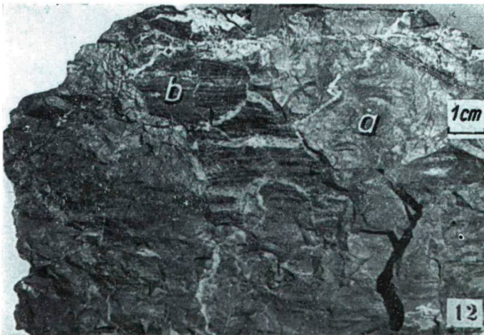
Fig. 12. Manganese oxide bank ( a ) oxidized from black, carbonate ore with remnant of the latter ( b ).
