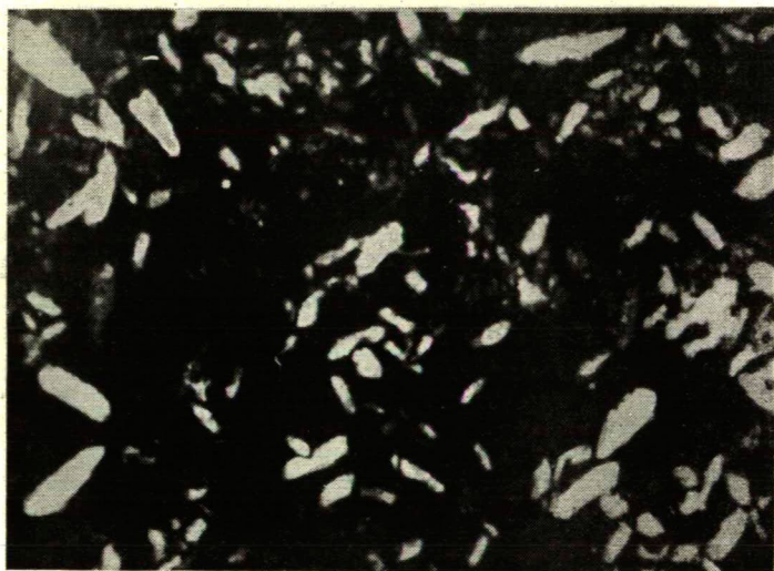
Fig. 6. Dickite crystals. Crossed nicols. 300 \times
