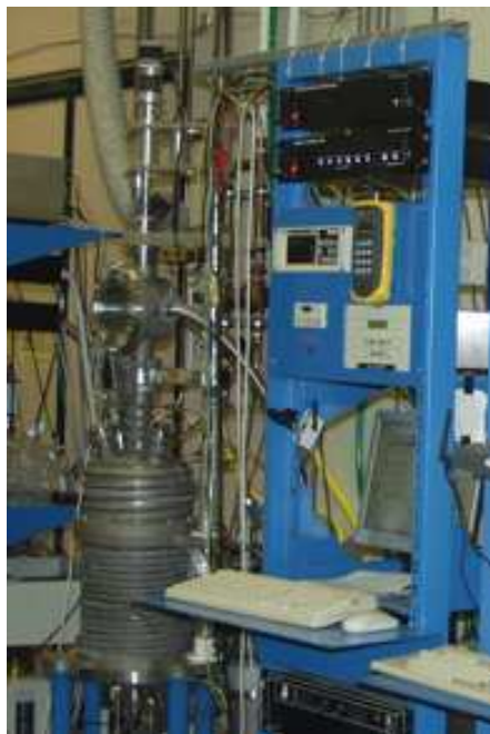
Figure 3.1: Czochralski furnace. - Czochralski growth apparatus at Pisa laboratory.
