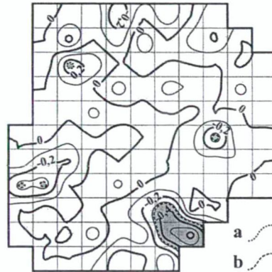
Fig. 3 The distribution of the difference between the annual mean maximum urban heat island intensity based on the complete database and based on the data of the selected 35 cells (April 2002 – March 2003), a - the upper limit of the confidence interval (0.25°C), (b) the lower limit of the confidence interval (-0.32°C)
