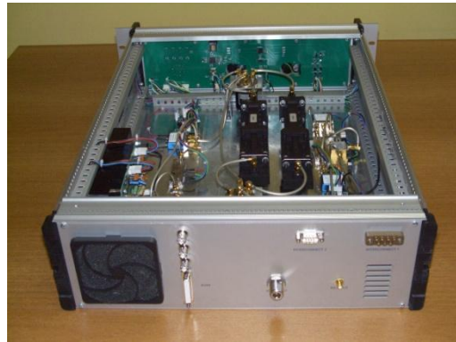
Figure 6.13 X-band RF receiver chain section 2; front (left) and rear (right)
