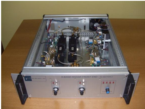
Figure 6.13 X-band RF receiver chain section 2; front (left) and rear (right)
