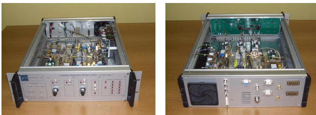
Figure 6.12 X-band RF receiver chain section 1; front (left) and rear (right)
