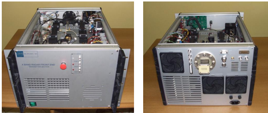
Figure 6.11 X-band RF transmitter chain front (left) and rear (right)
