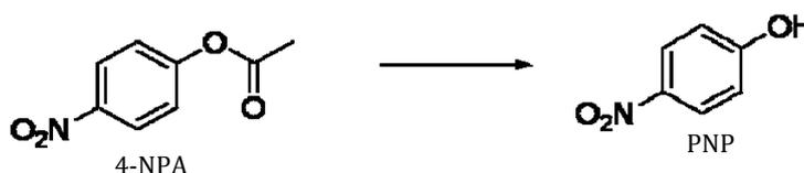
**Fig. 28.** Hydrolysis of 4-NPA and release of PNP.
