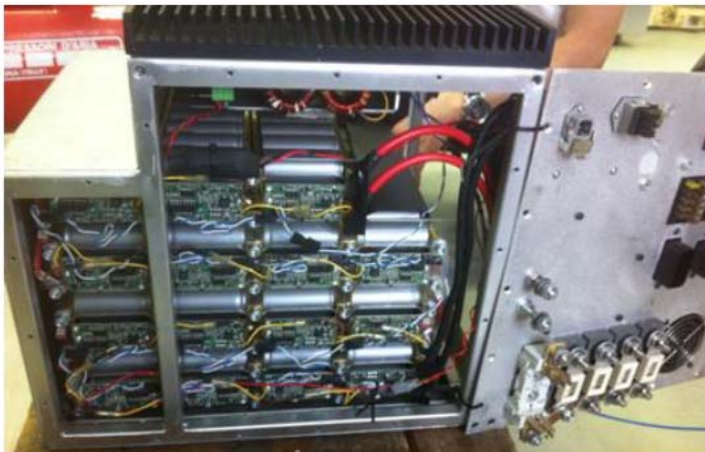
Fig. 1.12. Internal view of the PICAV battery for traction (DIME, 2012).
