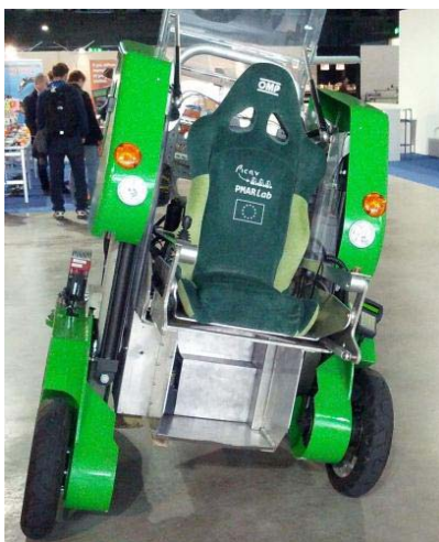
Fig. 1.13. The capability of the vehicle's wheels to allow the vehicle travel with two wheels in the sidewalk and two wheels on the road. Thanks to that, the user can be kept in a horizontal position (DIME, 2012).
