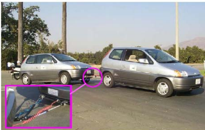
Fig. 2.8. The towing technique, in a mechanical way, through a tow-bar (Barth et al., 2004).
