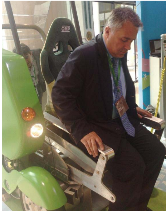
Fig. 1.14. The functionality of the seat. It accompanies the user when he raises and when he sits down, allowing mobility impaired people to sit and raise without using their muscles (DIME, 2012).
