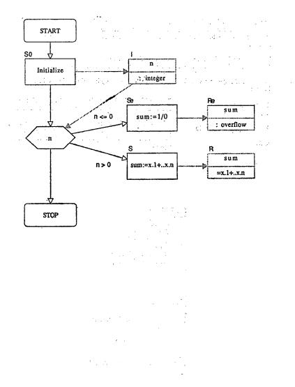
The refinement of the box S on the parent page is shown here. In the box S1 the initialization for the iteration is made and this makes the invariant P valid. The guard is given in box S2 and the variant n+1-i is shown at the end-of-iteration symbol.
