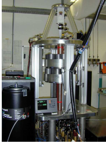
Figure 3.13: Picture of the mass holder and elevator. Two of the four legs are visible on the bottom; above them the reference horizontal plate and the four columns connected on the top by a circular plate. The two moving platforms are holding two sets of cylinders.
